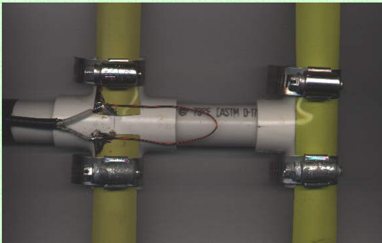
Figure 1. Close-Up view of RDF2 beam showing construction details
